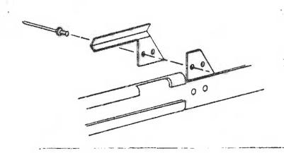
NOTE: Installation of Cockpit Vent Accessory Kit No. AK-113 includes installation of extended stops.
