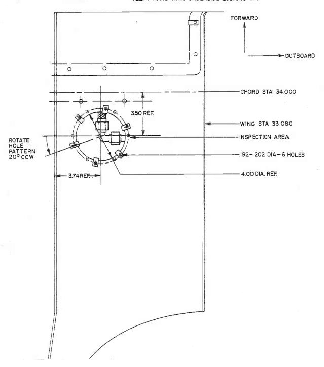
Figure 1. Wing Root Installation (Left-Hand Shown, Right Hand Similar)
